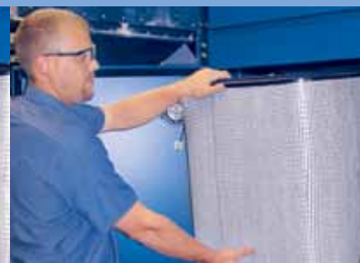
Filter is easily removed
